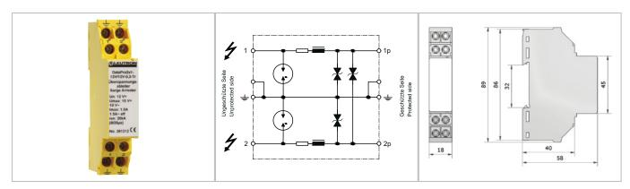
EMC filter for data and signal lines combined with surge protection enables smooth operation of sensitive electronic equipment in rough environment. Lightning current and surge voltage protection for particularly long signal and bus lines. Thanks to the extremely low volume resistance (impedance only  $0.3\Omega)$  no noteworthy signal losses occur. It is a combined arrester to protect two single wires. Applicable at the LPZ transition point 0A-1 and higher.
